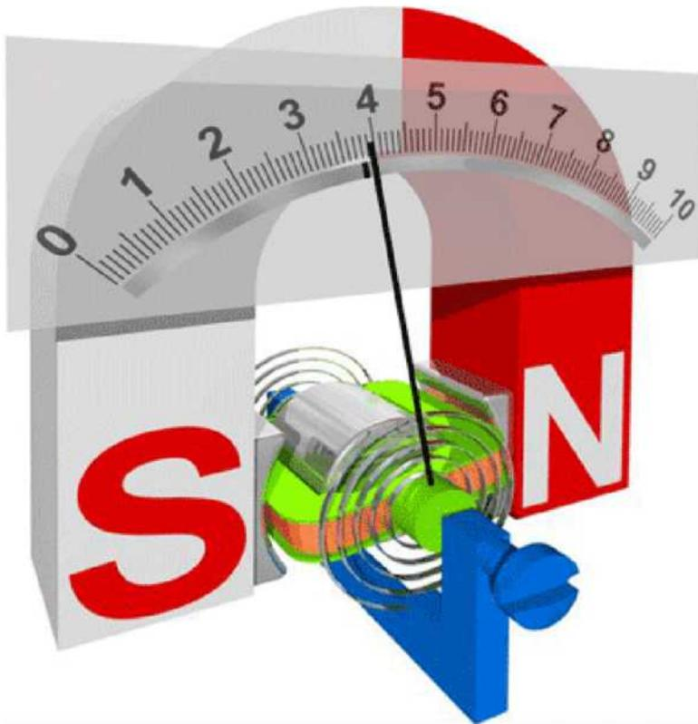
(a) **Stationary part or magnet system:** In the present time we use magnets of high field intensities, high coercive force instead of using U shaped permanent magnet having soft iron pole pieces. The magnets which we are using nowadays are made up of materials like alcomax and alnico which provide high field strength.
